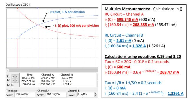
Figure 3.21: Multisim oscilloscope current measurements compared to calculations.
