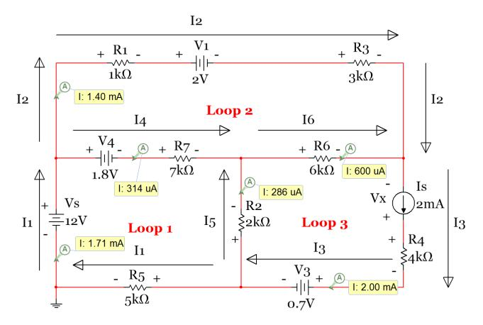
Figure 1.21: Circuit for Example 1.21
