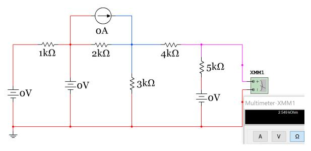
Figure 2.52: Multisim verification of Rth in Example 1.19 (done by plugging in zero for all sources instead of replacing with shorts and opens). This method is often easier to do quickly in Multisim.
