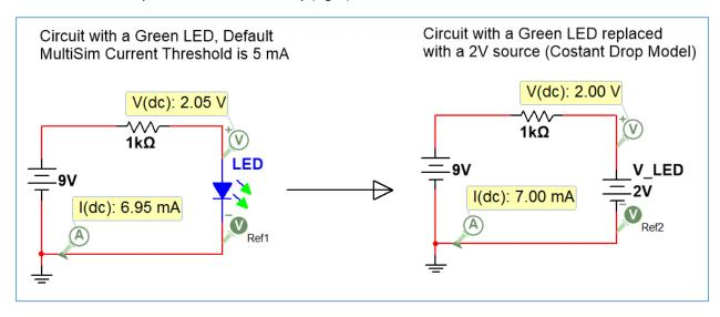
Figure 1.6: Example of a circuit with an LED in forward bias (left) and constant drop model (right).
