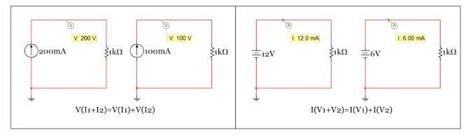
Figure 2.30: Example of an electrical component that is approximated to be linear – The resistor.
