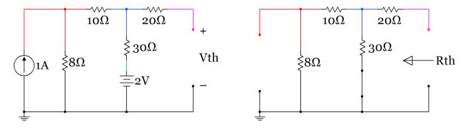
Figure 2.43: Sub-problem 1 (Find Vth – left circuit), Sub-problem 2 (Find Rth – right circuit)
