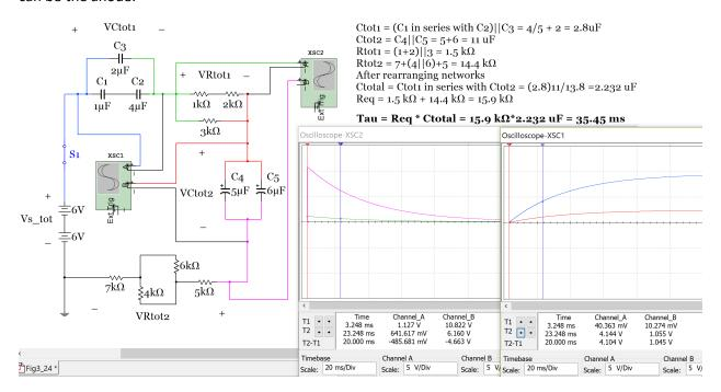
Figure 3.24b: Circuit for Example 3.8 and oscilloscope plots.
