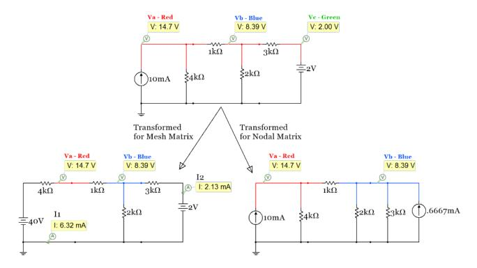
Figure 2.25: Circuit in <u>Figure 2.23</u> transformed to a circuit with only voltage (left) or current sources (right).
