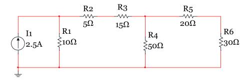
Figure 1.15: Circuit for Example 1.15
