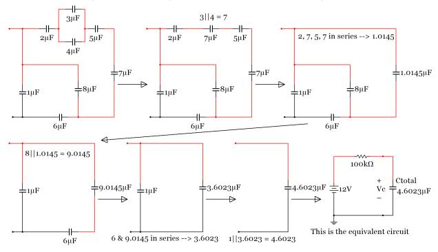
Figure 3.16: Determining Ctotal in Example 3.4
