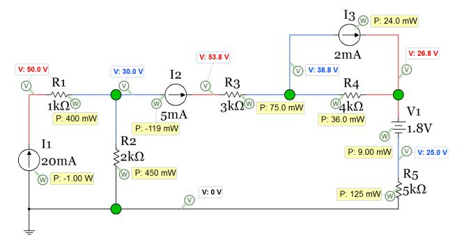
Find the voltage across I1 and I2 so power can be calculated.  $V_{11} = 50 - 0 = 50 \text{ V}$ ,  $V_{12} = 53.8 - 30 = 23.8 \text{ V}$
