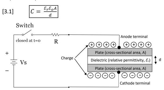
Figure 3.1: Illustration of a Capacitor connected to a battery and resistor (RC Circuit)
