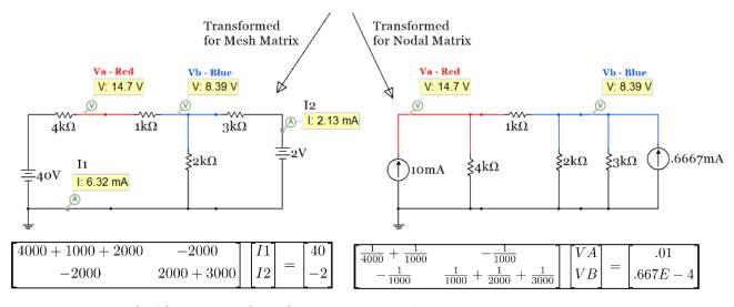
Figure 2.26: Mesh (Left) and Nodal (Right) Matrix solutions for Circuit in Example 2.11.
