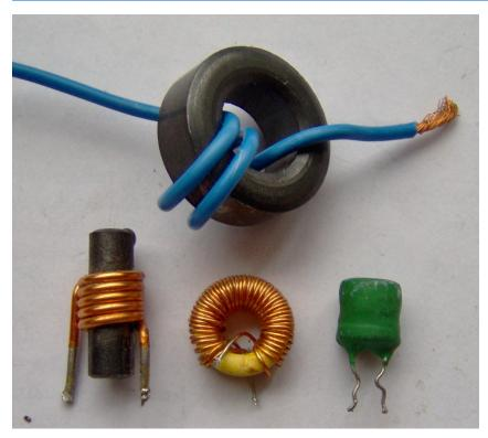
Figure 3.8: Inductor examples. Photo © FDominec and used under a CC BY-SA 3.0 license: <a href="https://commons.wikimedia.org/wiki/File:Electronic\_component\_inductors.jpg">https://commons.wikimedia.org/wiki/File:Electronic\_component\_inductors.jpg</a>
