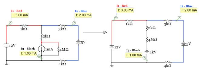
Figure 2.19: Circuit in Figure 2.18 with the virtual resistor added and transformation completed
