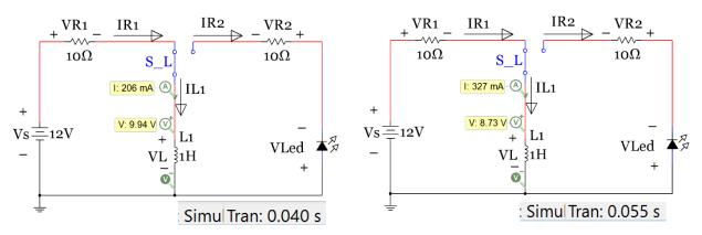
Figure 3.9: Store Circuit activated (Charging), 2 "moments in time" early in the charging process
