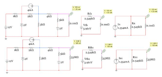
Figure 2.55: Demonstration that the Thevenin and Norton equivalent circuits produce the same results as the original circuit when connecting ANY resistor value to the Nubbies.
