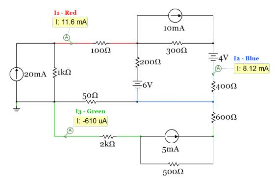
Figure 2.15: Circuit for example 2.8.
