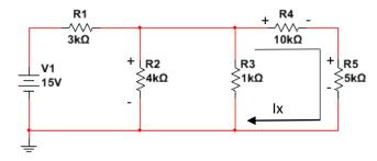
KVL: - I<sub>R2</sub> · R2 + Ix · R4 + Ix · R5 = 0 → - 0.7575 mA · 4 kΩ + Ix · 10 kΩ + Ix · 5 kΩ = 0 Ix =  $(0.7575 \text{ mA} \cdot 4 \text{ kΩ})/(10 \text{ kΩ} + 5 \text{ kΩ}) = 0.202 \text{ mA}$
