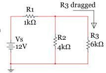
The <u>Guideline 6</u> sanity check states 2 resistors in parallel should give a result that is less than the smallest resistor (2.4 k $\Omega$  is less than 4 k $\Omega$ ) and if they are close to each other the result should be close to half the average (4k and 6k aren't "that close" to each other, but half the average is equal to 2.5 k $\Omega$  which is not that far off from 2.4 k $\Omega$ ).
