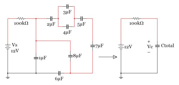
$C_{total}$  is found in a step by step fashion below. The most difficult part is visualizing that the 6  $\mu$ F capacitor is in parallel with the network that includes the 2  $\mu$ F, 3  $\mu$ F, 4  $\mu$ F, 5  $\mu$ F, and 8  $\mu$ F capacitors due to the tricky way it is drawn. The key to this step is that there are 2 connections (or they share 2 nodes), which is the definition of two components being in parallel. Another thing that could be done to help see this is
