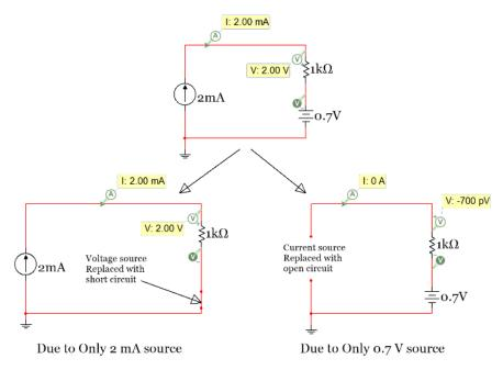
Figure 2.34: Example of Superposition with <u>Ideal</u> Sources
