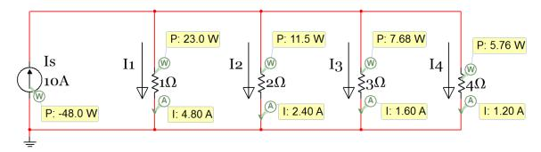
Figure 1.24: Circuit for Example 1.24
