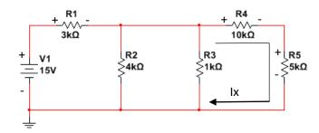
KVL: -15 + I<sub>S</sub> · R1 + Ix · R4 + Ix · R5 = 0 → -15 + 3.93 mA · 3 kΩ + Ix · 10 kΩ + Ix · 5 kΩ = 0 Ix =  $\frac{15V - 11.97}{10 kΩ + 5 kΩ} = \frac{0.202 mA}{10 kΩ + 10 kΩ}$
