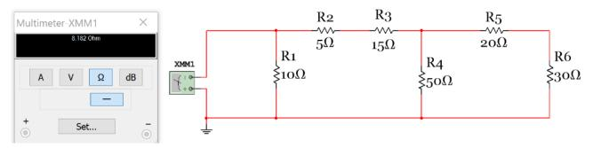
Step by Step solution to finding Rtotal.
