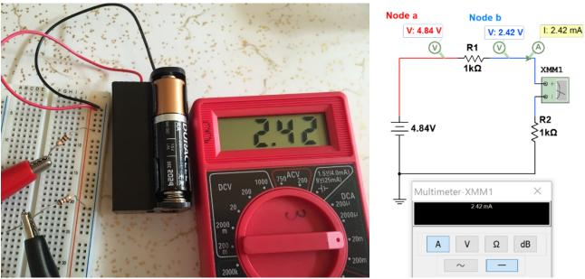
Figure 1.8: Circuit showing current measured with a Multimeter.
