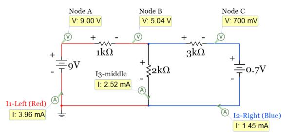
Figure 2.9: Circuit for Example 2.5 – The wires are color coded to match the currents instead of nodes.
