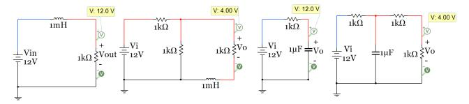
Figure 3.33: Passive Low Pass Filter (LPF) Circuit Examples
