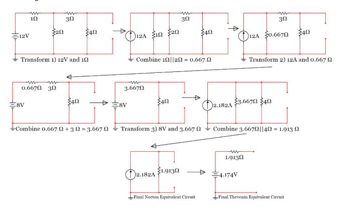
Figure 2.64: Finding Vth, I<sub>N</sub>, and Rth using Method 4 (Transform and Combine)
