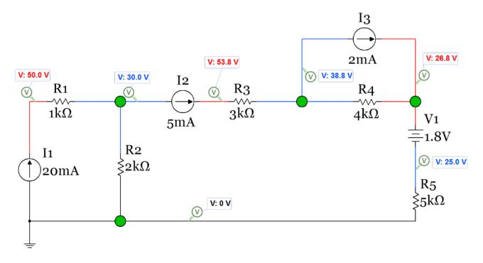
Figure 1.11: Circuit for Example 1.11
