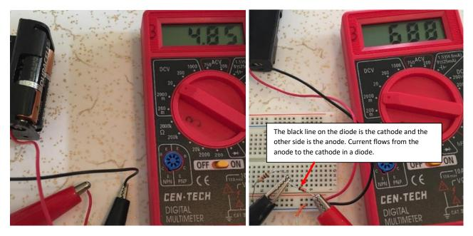
Figure 1.5: Multimeter voltage measurements of a battery pack (left) and 1N914 Diode (right)
