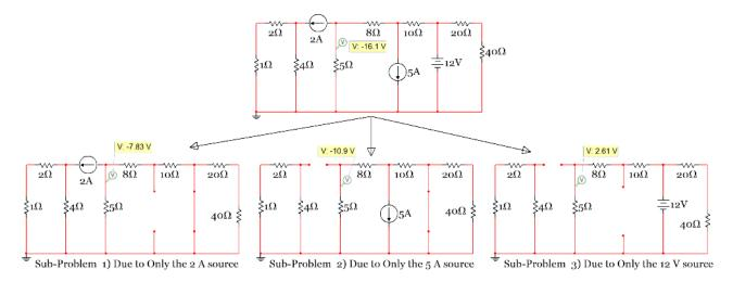
Figure 2.38: Circuit for Example 2.17
