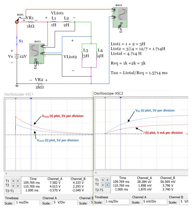
Figure 3.23: Circuit for Example 3.7 and oscilloscope plots.
