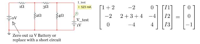
Figure 2.63: Sub-Problem 2 - I<sub>Test</sub> Calculation - Used in Method 3 to determine Rth = V<sub>Test</sub>/I<sub>Test</sub>)
