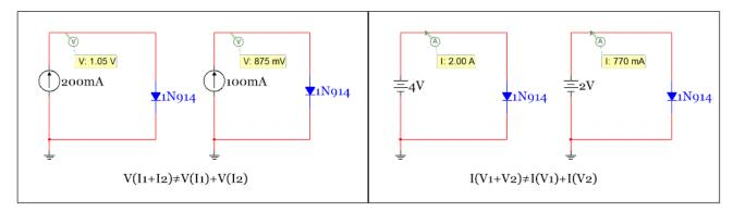
Figure 2.31: Example of an electrical component that is <u>extremely non-linear</u> – The diode.
