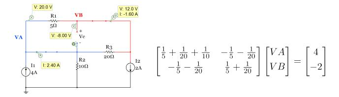
Figure 3.28: Circuit in Example 3.10 redrawn and nodal matrix solution
