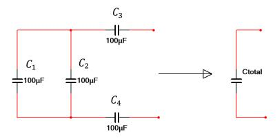
Figure 3.13: Combining capacitors for example 3.3.
