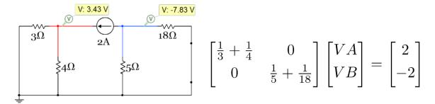
Figure 2.39: Circuit and Nodal Matrix equation for sub-problem 1 of Example 2.17
