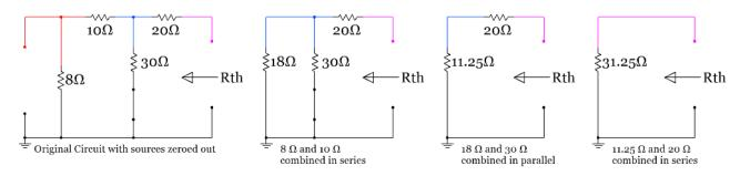
Figure 2.46: Step by step solution for calculating Rth in Example 2.18
