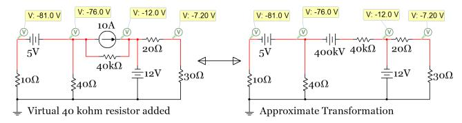
Figure 2.8: Approximate Source Transformation of Circuit in Example 2.4
