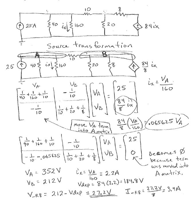
The following handwritten example shows how to do Mesh Matrix with a dependent source.
