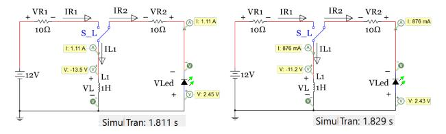
Figure 3.10: Release Circuit activated (Discharging), 2 "snapshots" early on in the discharging process
