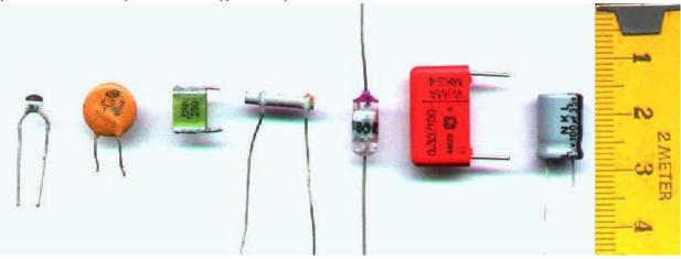
Figure 3.2: Different types of capacitors. From left: multilayer ceramic (MLCC), ceramic disc (see <u>Figure 3.3a</u>), multilayer polyester film, tubular ceramic, polystyrene, metalized polyester film, aluminum electrolytic. Photo © aka and used under a CC BY-SA 3.0 license.
