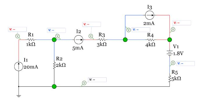
Figure 1.10: Circuit for Example 1.10
