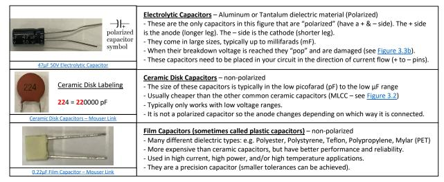
Figure 3.3a: Description of three of the most common types of capacitors.
