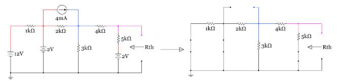
Figure 2.49: Sub-problem 1 circuit with sources replaced with shorts and opens (or "zeroed out")
