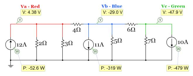
Figure 2.29: Circuit for Example 2.15
