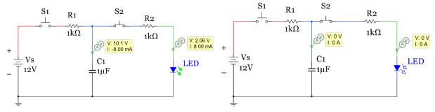
Figure 3.5: Discharging a Capacitor across an LED (Left – barely discharged, Right – fully discharged)
