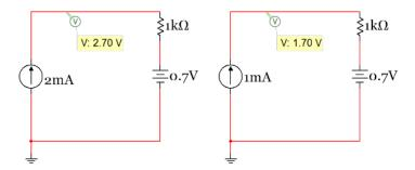
Figure 2.32: Example of a <u>linear system</u> - Circuit with a resistor and a diode that is replaced with a battery.
