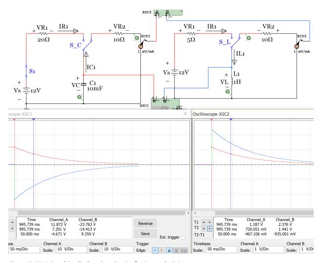
Figure 3.25: RC and RL discharging circuits for Example 3.9.
