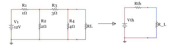
Figure 2.57: Circuit used to show the 4 different methods of finding the Thevenin Equivalent Circuit
