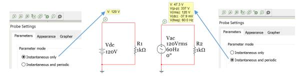
Figure 1.7a: Preferred probe settings for DC circuits (Left) and AC circuits (Right).
