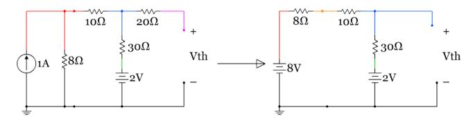
Figure 2.47: Original circuit (left) set up for finding Vth and transformed/simplified circuit (right)
