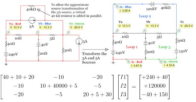
Figure 2.28: Circuit and Matrix for Example 2.14
