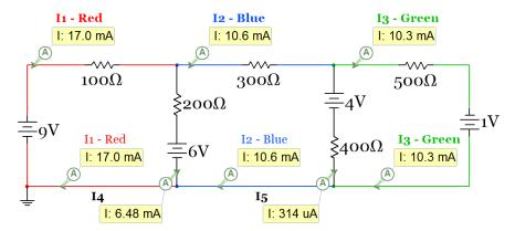
Figure 2.13: Circuit for example 2.7.
