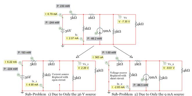
Example 2.16) solve the following circuit for the voltage and current labeled  $V_x$  and  $I_x$  using superposition.
