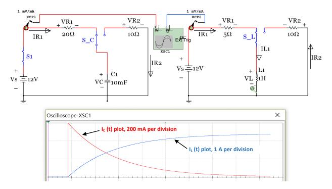
Figure 3.20: Multisim oscilloscope plot for the current in the RC and RL charging circuits.
