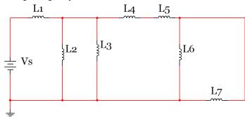
Using equation 3.6 and the provided information (I = 0.1 m, N = 100 turns,  $\mu_{r\_iron}$  = 100,  $\mu_{r\_iron}$  = 1.2566370614×10<sup>-6</sup> kg·m/A<sup>2</sup>·s<sup>2</sup>, and A =  $\pi$  (0.03)<sup>2</sup>/4 = 7.0685E-4 m<sup>2</sup>. the value of the inductance for each inductor can be found.
