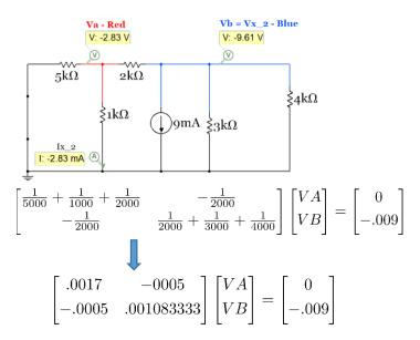
Figure 2.37: Circuit and Nodal Matrix equation for Sub-Problem 2 of Example 2.16
