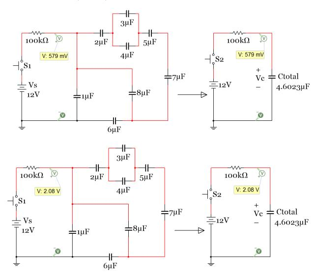
Figure 3.18: Example 3.4 Multisim verification
