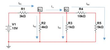
Figure 1.22: Circuit for Example 1.22
