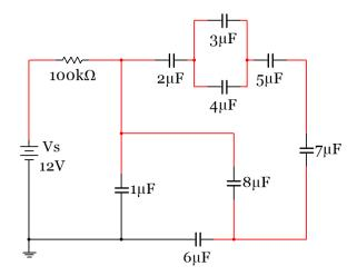
Figure 3.15: Circuit for Example 3.4.
