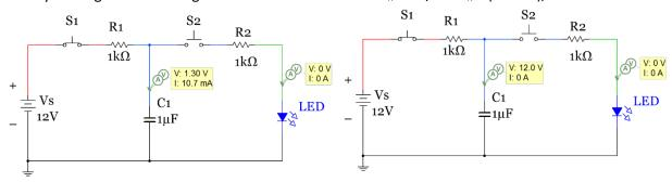
Figure 3.4: Charging the Capacitor in a RC circuit (Left – slightly charged, Right – fully charged)
