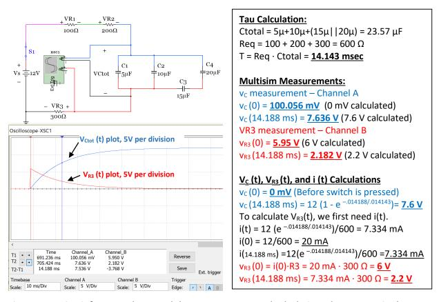
Figure 3.22: Circuit for Example 3.6 and the measurements and calculations that are required.
