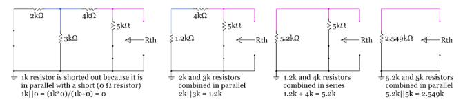
Figure 2.50: Step by step solution for calculating Rth in Example 2.19
